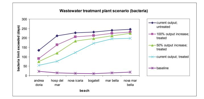
Releasing the treated effluent away from the beaches (baseline) has a significant effect especially to the nearest beaches (nova mar bella). Increases in output of effluent also significantly negatively affect the water quality.
