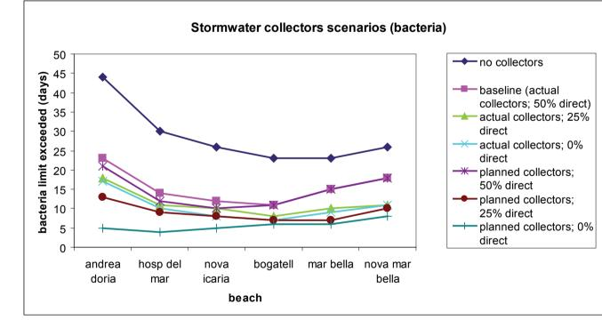
Both the percent of CSO directly released and the capacity of storm water collectors have a shared effect in reducing days in which bacteria limits are exceeded.
