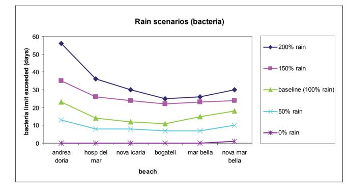
In contrast to the effect rain has on suspended matter, days in which the bacteria limit is exceeded almost disappear when there is zero precipitation. Increased rain affects each beach approximately the same, with those nearest to the river least affected.
