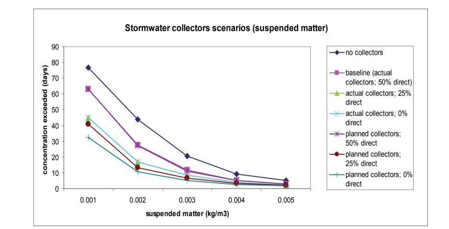
Increased rain has a greater affect on low concentrations of suspended matter than on high concentrations. Even with zero rain, days with lower concentrations of suspended matter are still fairly frequent (produced by wave re-suspension and the river).
